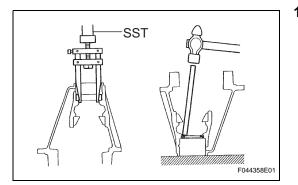
(d) Remove the rear differential case assembly from the differential carrier. HINT:
